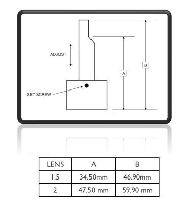
Measurement "A" is the critical dimension and should be used in the first instance.
