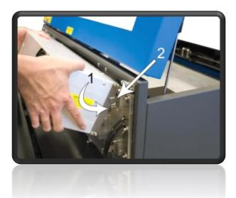
5- Pick up the laser cartridge by the ends and tilt it at a 30 degree angles as shown (1). Mount the laser cartridge onto the mounting blocks shown in step 2 by placing the upper "V" groove on top of the mounting blocks.
