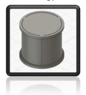
The side panels are to be 3D printed, for which you can follow the normal printing procedures for your brand of 3D printer. The top and base are to be laser cut. As you can see they are not a 2D representation of what we require to enable use in a Universal Laser.
